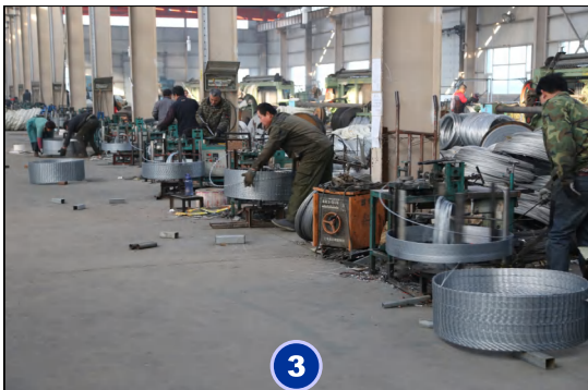
Wrapping the Wire with Blades
